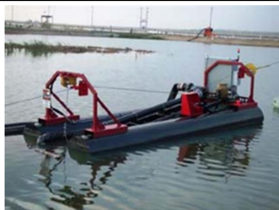
Figure A6.5: Dredging system for WSPs
