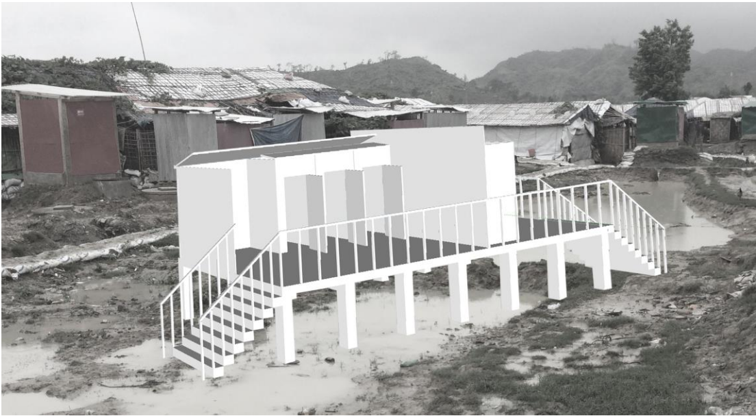
Figure 8: bathing and laundry facility in flood prone areas; note that the bannisters are solid walls, but have been removed to allow internal visualisation.
