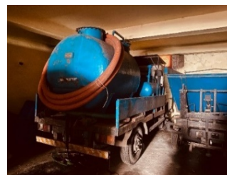
Figure 2 : Desludging vehicle used for emptying of OSS (Source: Sachin/NIUA/2024).
