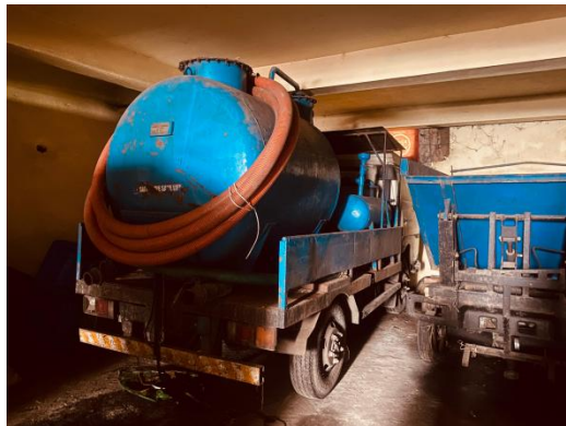
Figure 13: Desludging vehicle used for emptying of OSS (Source: Sachin/NIUA/2024).
